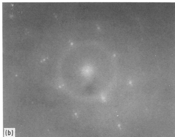
Figure 2 (a) Bright-field image of the film implanted with 170 keV \text{P}^+ at a dose of 5 \times 10^{15} \text{ cm}^{-2} showing that the amorphous zones were formed in the 2212 grain. (b) Diffraction pattern of (a).
